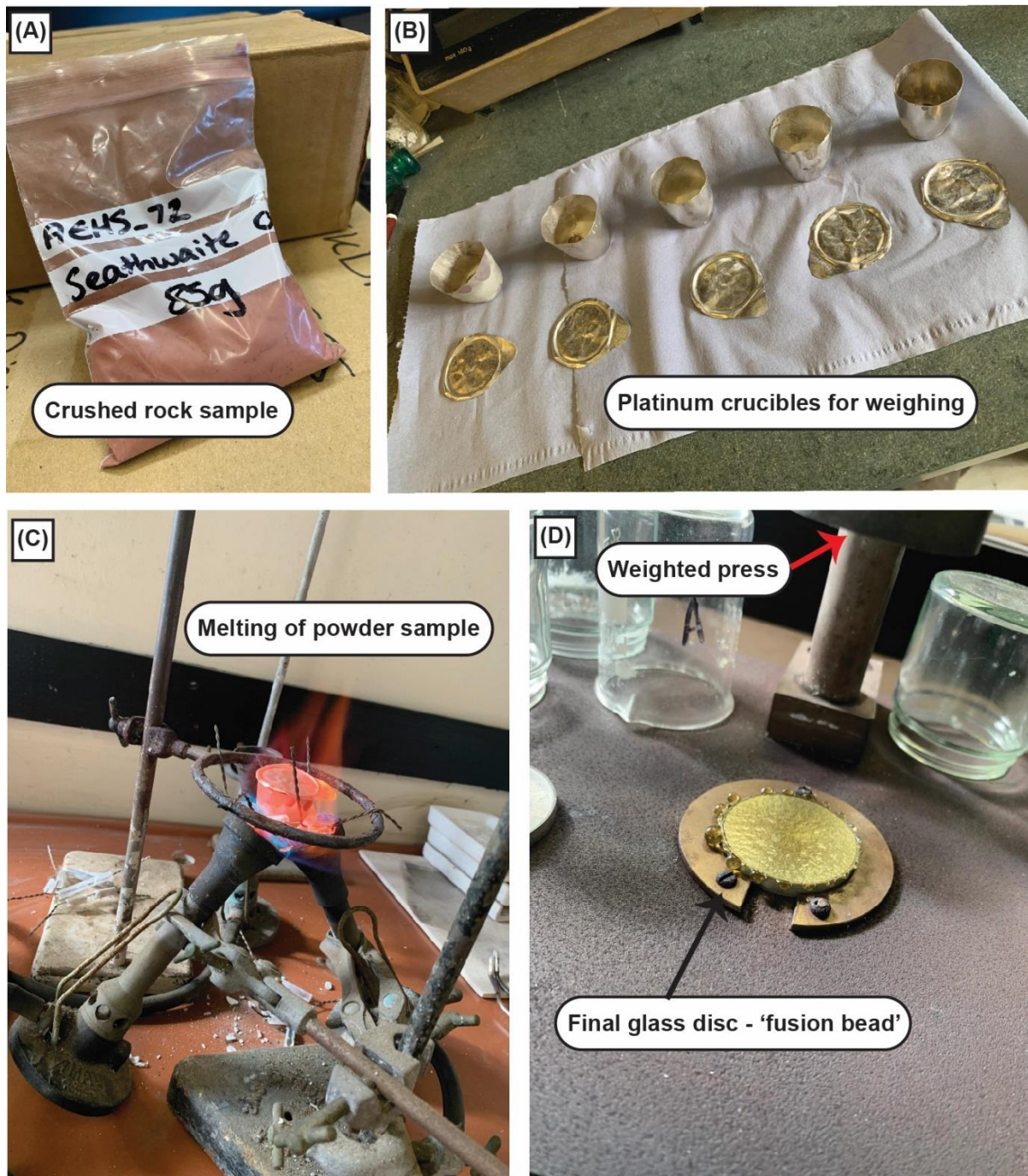
Figure 2: (A) Crushed rock sample from Seathwaite; (B) weighing stage of the process, putting sample into platinum crucibles; (C) melting of sample within the crucibles into a molten glass; (D) pressed molten glass onto Al-disc, creating the final fusion bead.
